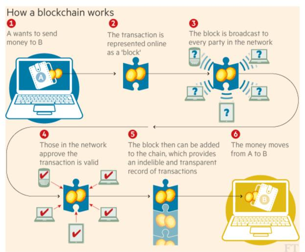
Figure 4 How a Blockchain works (http://technofaq.org/posts/2016/08/blockchain-what-is-it-and-how-can-we-use-it/)
